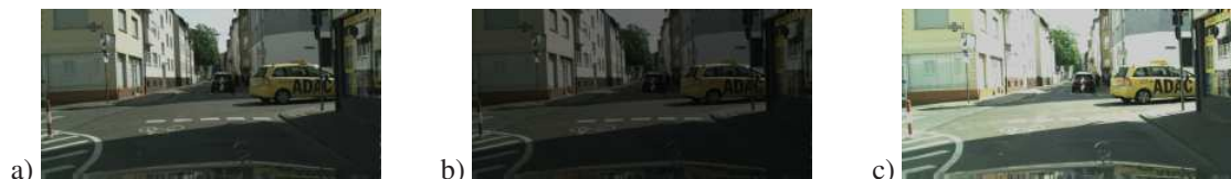
Figure 3: Contrast modification on a Cityscapes validation image; a) original image; b) c = 0.5 ; c) c = 2
