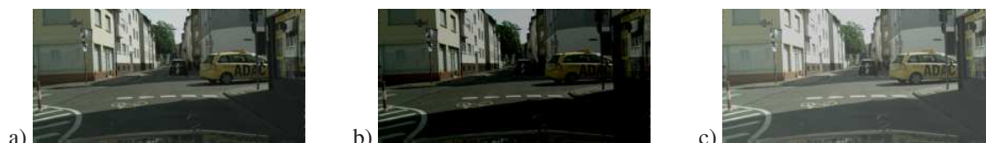
Figure 2: Brightness modification on a Cityscapes validation image; a) original image; b) b = -50 ; c) b = 50
