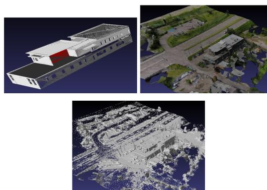
Figure 15: The CAD model of the building (a), the real area of the building (b), the large-scale point cloud of area (c).
