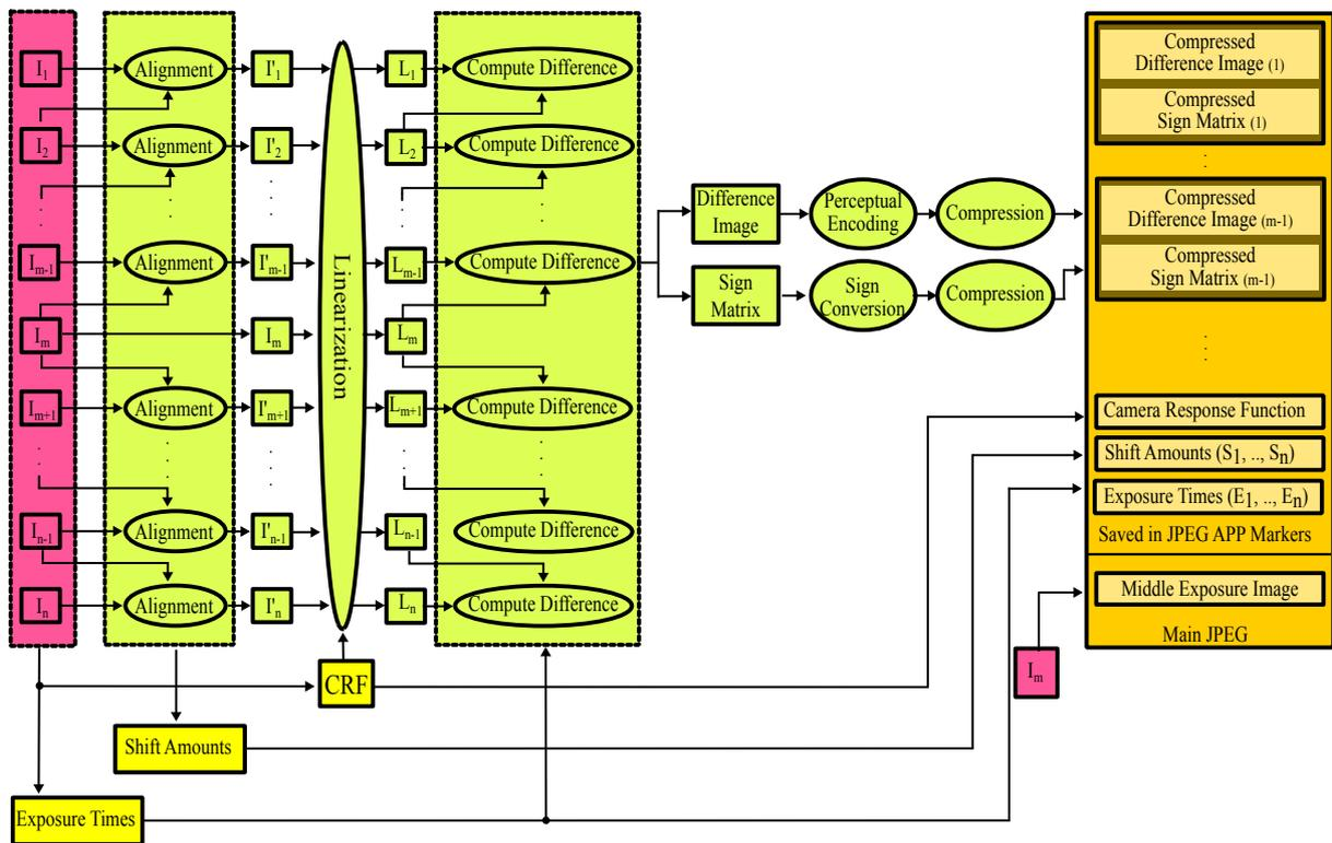
Figure 1: The compression pipeline of the CES algorithm.
