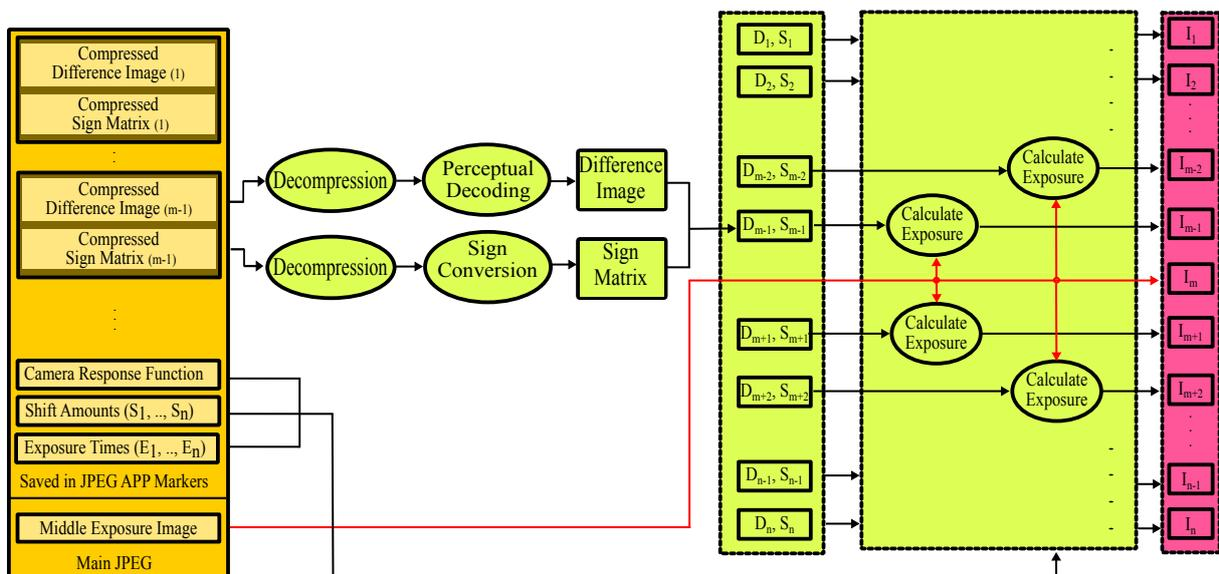
Figure 2: The decompression pipeline of the CES algorithm.
