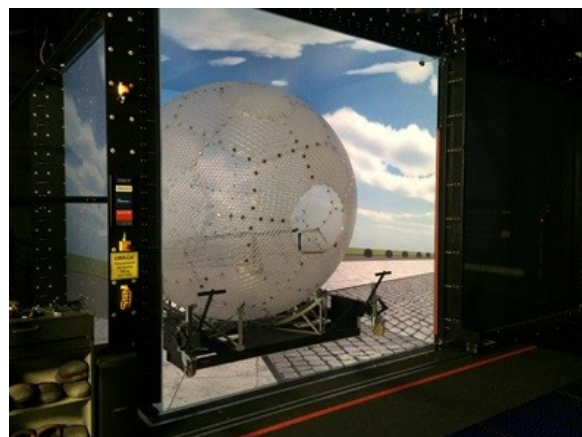
Figure 2. Spherical walk simulator in the middle of VR cave in I3DVL (with open gate).
