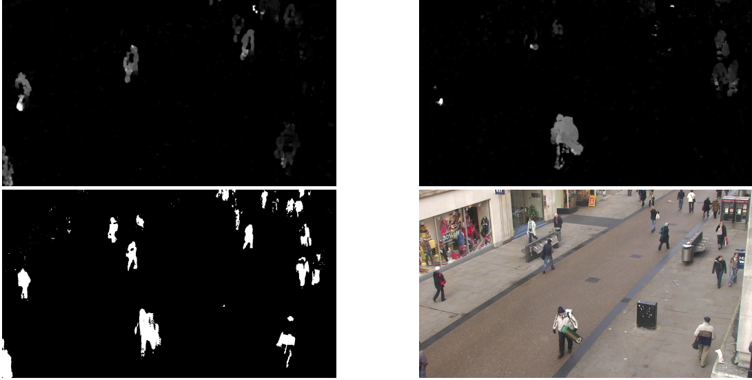
Figure 1: In the top row the intensities of the optical flow are depicted for an image. On the left side for the right-left movement and on the right for the up-down movement. In the bottom row are the original frame from the video and the segmentation result.
