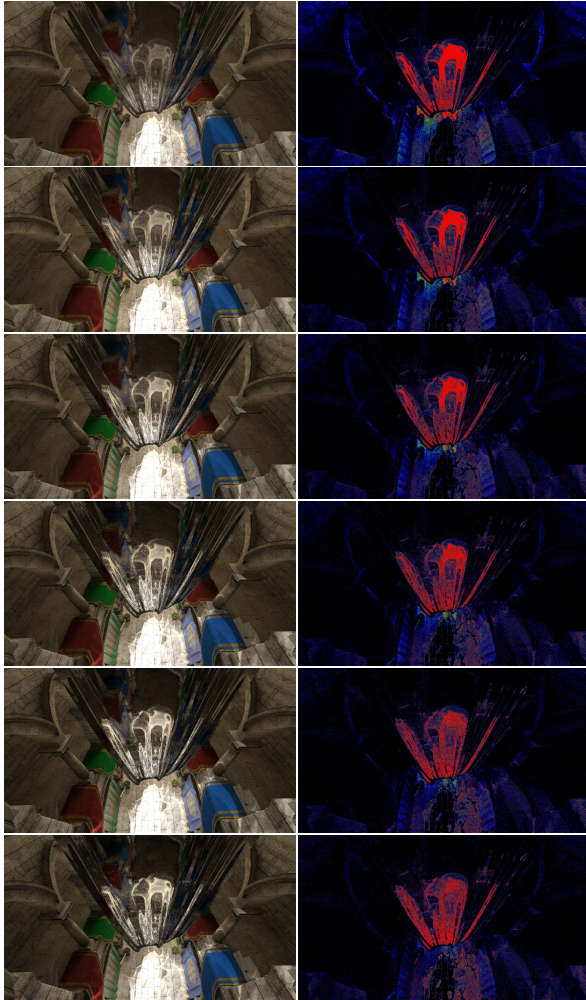
Figure 9: Sponza view 2 with different speculative tree depth d increasing from 1 (naive) to 6. All images were generated in 10 minutes on the GeForce GTX Titan.
