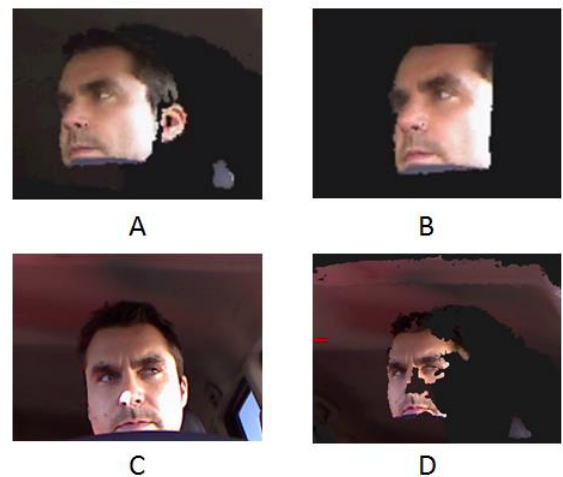
Figure 5: Examples of normal face detection (A and B) and error due to extreme light conditions (C and D).
