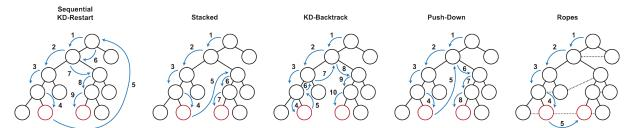
Figure 2: Traversal order example for different KD-Tree Traversal algorithms. The red circles represent two leaf nodes that, must be traversed in order. The main difference between KD-Tree traversals is how they go from the red circle to the other. The dashed lines represent the ropes.
