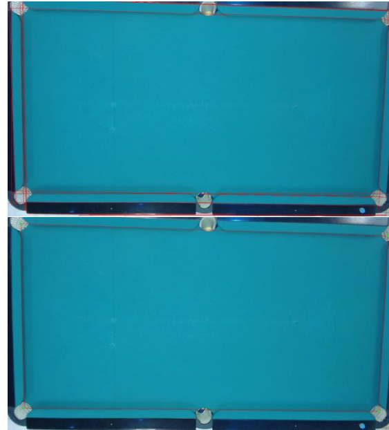
Figure 3. Top, detected lines and in the bottom final automatic table boundaries extraction.
