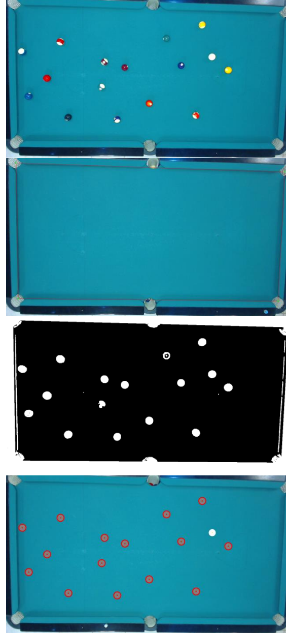
Figure 5. Top to bottom, A_t , the reference frame E , the subtracted binary image from the above images Fgb_t and the images with the detected balls in red, plus the white.
