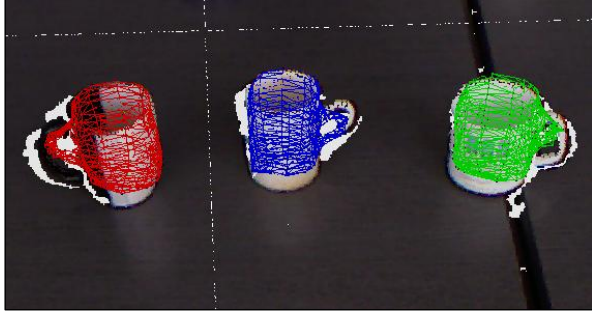
Figure 1: Full 3D volumetric reconstruction of multiple objects in a mobile manipulation scenario.
