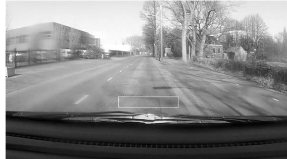
Figure 2. Picture taken with an onboard camera. The region of analysis is indicated by the white box below the center of the image.
