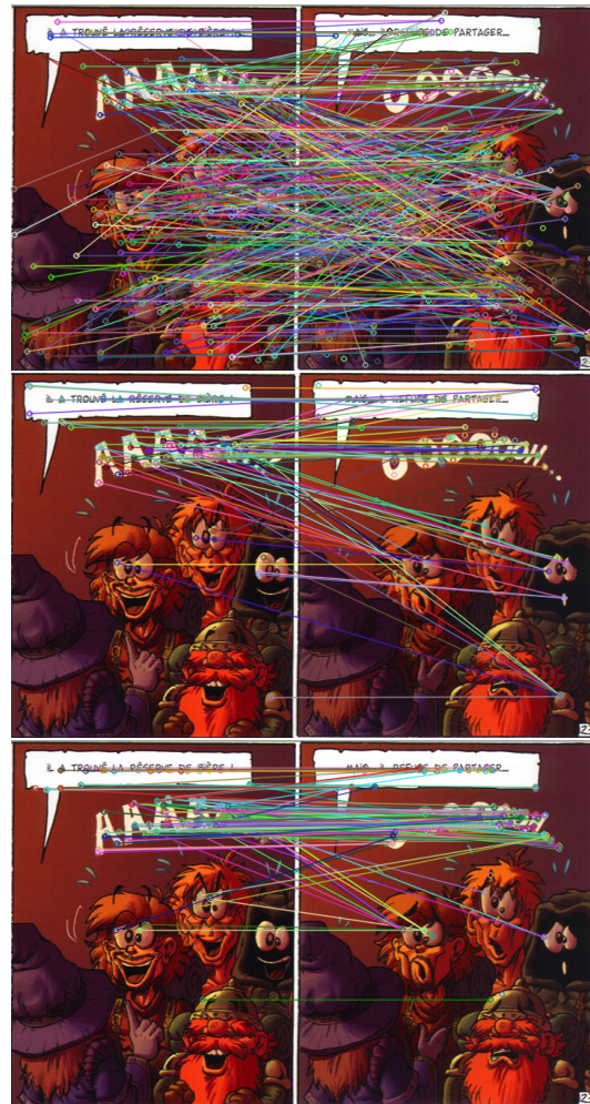
Figure 7: Up to down: SIFT, SURF and ORB detectors on two panels of comic Le Donjon de Naheulbeuk .
