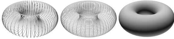
Figure 6. Different display modes: points, wireframe and solid.
