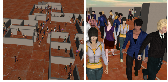
Figure 6: This figure shows two images of an office evacuation crowd scene with two hundred articulated characters. This scene consists of 16.4 M triangles. Our method can achieve 49 frames per second (fps) on average for this scene.
