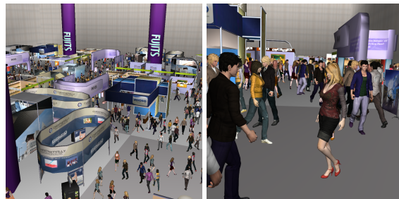
Figure 1: This figure shows two images of an exhibition crowd scene that has 1 K articulated characters. All the characters and the scene have 83 M triangles. Our method achieves 46 frames per second (fps) on average for this model with 0.5 pixel-of-error (PoE) in a 1280 by 720 HD screen resolution.
