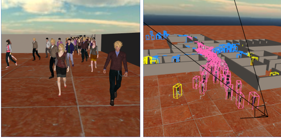
Figure 9: The left figure shows the image created at a first person view. The right image shows a third person view with occlusion results. The black lines show the view frustum of the first person view. The pink, blue, and yellow boxes are visible, occlusion culled, and view-frustum culled clusters.
