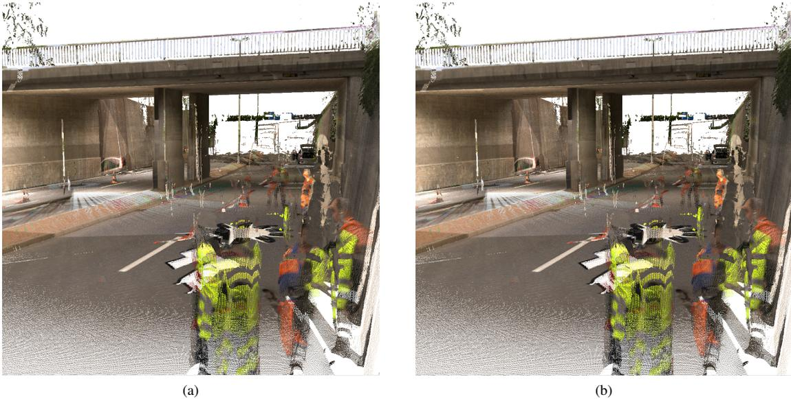
Figure 4: Comparison of (a) OpenGL rendering and (b) OpenCL rendering. As one can see, rendering results are almost identical. There are only small differences in far away parts of the scene, because we use eight bits more depth buffer precision than OpenGL. While the OpenGL version runs at about 5 frames per second, our implementation reaches 56 fps.
