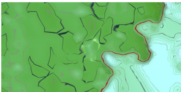
Figure 3 Procedural contour lines in a shallow wetland area, as-is and using a 'gradient compensation' exponent of 16 to narrow lines.
