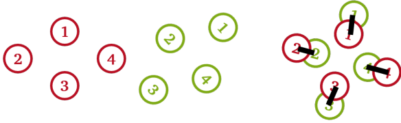
Figure 3: Rotating one of the two point clouds (green) reduces the average distance between pairs.
