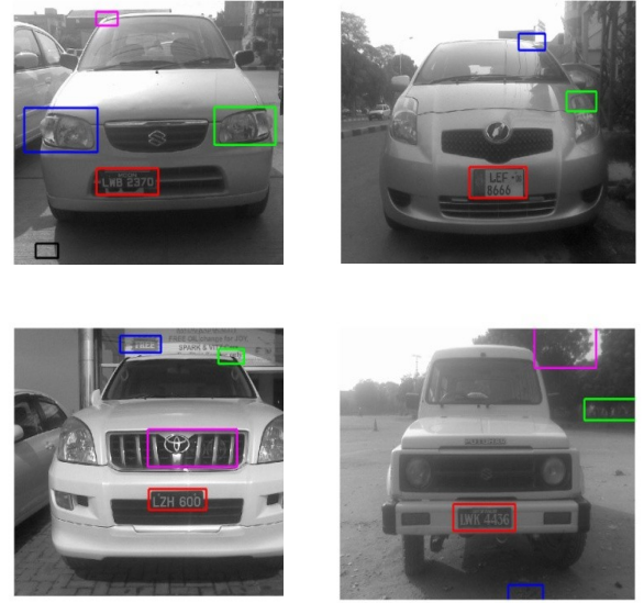
Figure 1. Examples demonstrating the connected components found in the images, where Red rectangular bounding box represents true localization of license plates.
