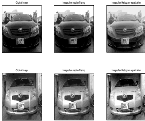
Figure 6. Representing the first phase of the algorithm, where standard pre-processing techniques are applied to increase image quality. First Column contains Original input images, Second Column contains images after removing salt & pepper noise, Third Column is representing image after contrast enhancement.
