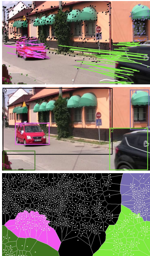
Figure 4. Motion segmentation of scene with two moving cars. From top: tracks, bounding boxes, Voronoi tessellation of the whole image.
