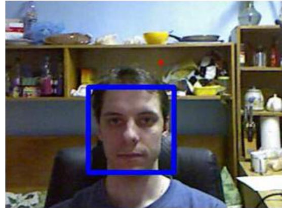
Figure 2. Face tracking. Kinect detects face by using Haar classifier included in OpenCV library. In the next step, pan/tilt motors adjust Kinect position such that the face rectangle is in the center of image.
