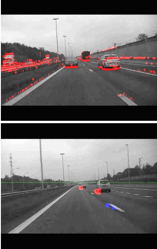
Fig. 1. Result of single-frame analysis with different settings of darkness criterion and brightness drop-down. Candidate cars have been marked red; white lane markers marked blue; the assumed horizon is represented by the green line (bottom).
