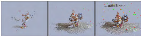
Figure 4: Several SfM stages of the reconstruction of our Rooster dataset. Left: the initial two-frame reconstruction. Middle: an intermediate stage after 20 images have been added. Right: the final construction with 42 images.
