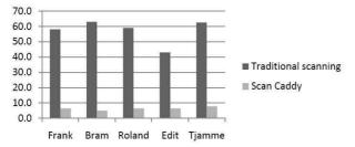
Figure 9 Time (in minutes) it took test persons to carry out a 3D scanning process with and without supplying the FOB data. The FOB facility was called Scan Caddy in the particular experiment.
