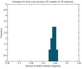
Figure 7. Spread of the intrinsic rotation  $\theta_X$  for arbitrary measurements (top) and mechanically identical measurements (bottom).
