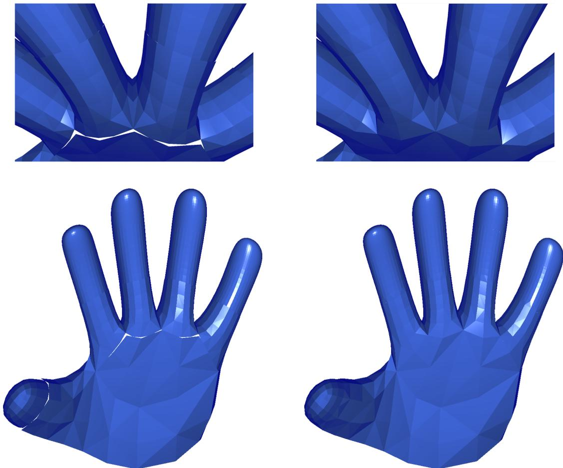
**Figure 17: Hand model at different LODs. Left: without junction adjustment, right: with forced border vertices.**
