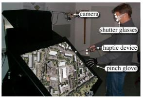
Figure 5. Workbench environment with an optical tracking system.
