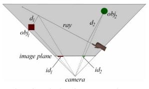
Figure 3: Projection of world space distance vectors onto the image plane.
