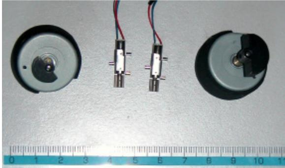
**Figure 5. The Wingman vs SenStylus rumble motors.**
