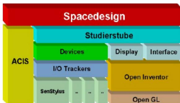
**Figure 2. The Spacedesign VR CAD application architecture.**
