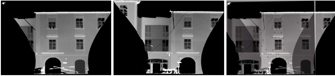
(a) (b) (c) Figure 3: Orthogonal rectified range image pair and registration result: (a) right image. (b) left image (c)Registration result for the range image pair. The corresponding points are shown as black crosses.
