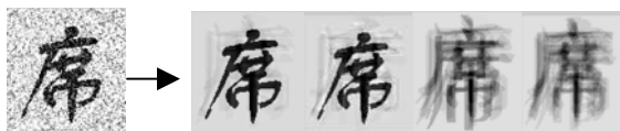
Fig 7: De-noising images by linear PCA (first is noised image, next four with principal components of 11, 9, 4, 1 respectively)
