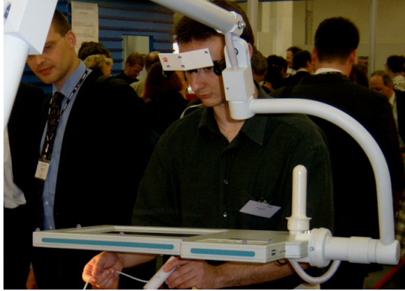
Figure 2. Glasses and transparent display, both equipped with infrared markers.
