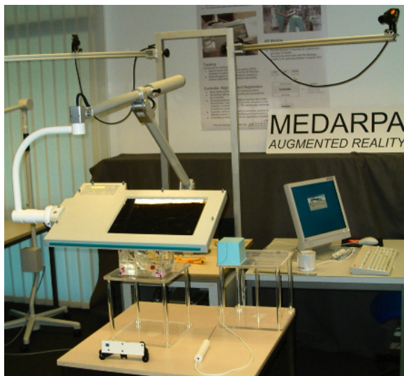
Figure 1. Augmented Reality System for minimal invasive surgery. Infrared cameras track the AR display. Eyeglasses and instrument are lying on the table.
