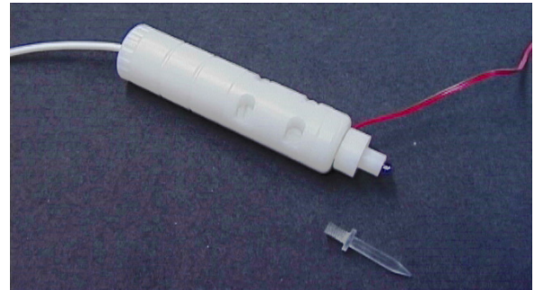
Figure 3. The alignment device with integrated electromagnetic sensor and additional infrared diode on tip.
