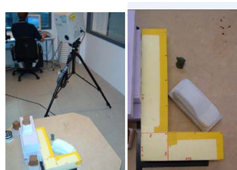
Figure 3. Workpieces have been placed on the platform, near the L-shaped reference object P . A top view is shown on the right. Both test objects A_1 and A_2 are shown, a small (2cm diameter) puppet and a 25cm car model, respectively.
