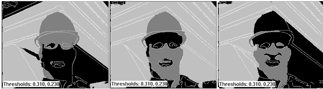
Figure 4. Region motion and order computed from boundary motion for three successive frames. Light gray regions are those unambiguously assigned to the background and dark gray regions are unambiguous object regions. Black regions are ambiguous and, depending on the actual labeling, can be either background or foreground. As explained in text, conflict regions are also treated as ambiguous.
