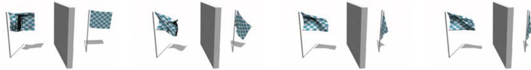
Figure 4: Two flags blowing in the wind (Navier-Stokes equations). The wind is blocked by the wall, so the right flag is in the lee. Note that the simulation starts with both flags in an unfolded state.
