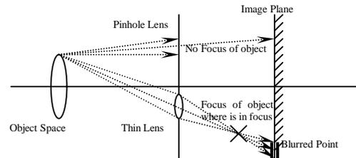
Figure 3. Infinitely small pinhole and thin lens.
