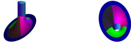
Figure 10: Conversion of a blending scaled cyclide into three RQB surfaces
