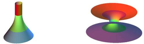
Figure 11: Left. cylinder-cone blending. Right. cone-cone blending
