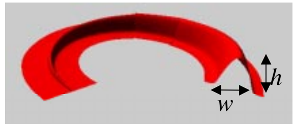
Fig. 6. Top: The series of 20 straight ridge templates making up the total feature structure. Bottom: The 19 features are merged as to form a single FFF, controllable with two design parameters, h and w .
