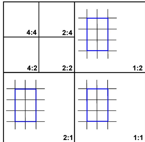
**Figure 3. Multiresolution decomposition in JPEG2000 using different scaling values (blue: subband areas belonging to a single precinct).**
