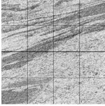
**Figure 4. Division of a non-homogenous rock sample into 16 blocks.**
