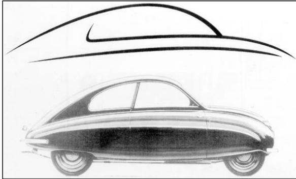
**Figure 2. Examples of characterising curves (Courtesy of SAAB).**
