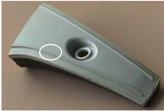
Fig. 1. Test object A was digitized to generate the data points s_i . The feature of interest in this object is formed by the longitudinal ridges in the upper surface. The white ellipse indicates the region containing the data representing the shape S .
