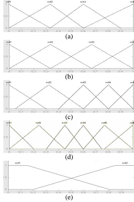
The membership functions for all variables. (a, b, c, d, e) The membership functions for  $x_1, x_2, x_3, x_4$  and  $y$ , respectively
