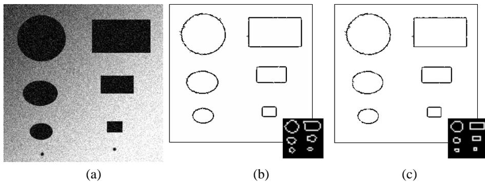
A Gaussian noise contaminated synthetic image to verify the effect of the proposed method with different edge detection methods applied on top level of MP. (a) The original image. (b) The initial edge map on top level with Sobel edge detector and the final edge map on bottom level. (c) The initial edge map on top level with thresholding method and the final edge map on bottom level.
