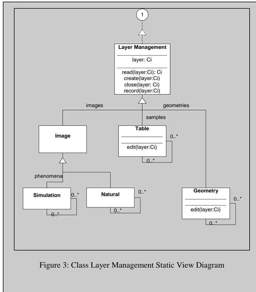
Figure 3: Class Layer Management Static View Diagram
