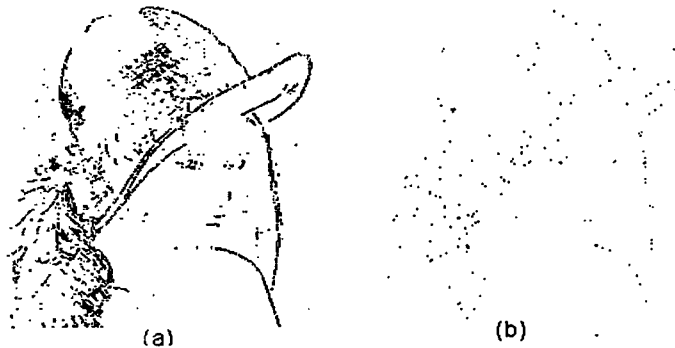
Fig 8. The gradient magnitude picture of the standard "Lena" photograph has been computed. (a) The gradient has been fuzzy windowed relative to [128,128]; (b) the same gradient windowed relative to [128,128].
