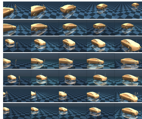
Figure 3: Visualization of collision simulations (rows). All subjects were represented with both actions, utilizing a single-car model for consistency. (left) Initial frame (right) Last frame
