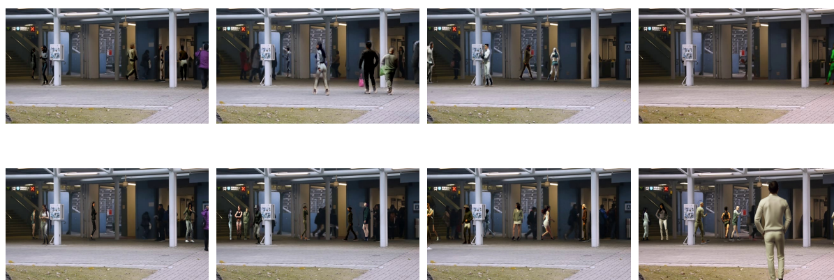
Figure 2: Examples of anonymized frames using the proposed pipeline, where the generative model only uses skeletonizations and masks.
