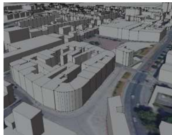
Figure 2. 3D model of the center of Zlín in Blender acquired by Blender GIS script
