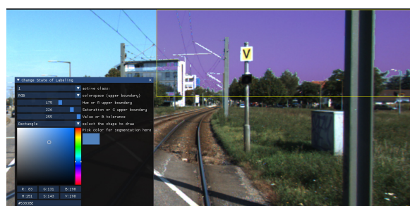
Figure 2: Applying a Threshold to segment the region "sky".
