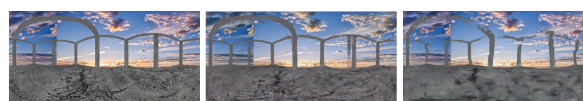
Figure 7: The figures illustrate the rendering of the first scene at the point, which was not part of the training set. The first image is the real image at that point, the second is the prediction of the first CNN, and the third is the image predicted by the second CNN.
