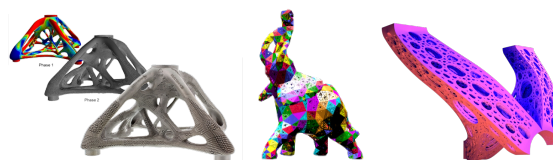
Figure 1: Left: Example of a topological optimization with two levels of lattice structures (©Altair Engineering). Middle: Elephant structure (from CGAL Computing Library at https://github.com/CGAL/cgal ) built with multi-scale lacunas. Right: part of a mechanical system redesigned with multi-scale lacunar components shown in Figure 2.
