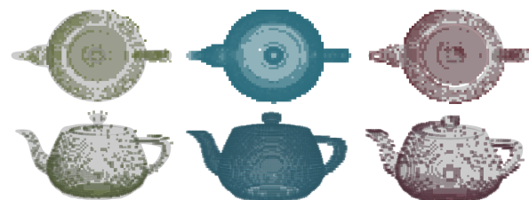
Figure 9: In the top row contains an overlay of the difference set B_d \setminus A_d (yellow), the intersection set A_d \cap B_d (blue) and the difference set A_d \setminus B_d (red) with transparent digital twin from above using a orthographic projection. In the bottom row, the same sets are rendered on top of the transparent 3d object from the side using a perspective projection.
