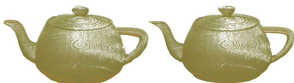
Figure 11: Difference sets A_d \setminus B_d (left) and B_d \setminus A_d (right) resulting at a dense voxel size of 0.25mm (fourth run of the second object in Table 3). In addition, the color gradient is used to illustrate the strength of the deviations.
