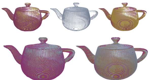
Figure 12: Top row: difference A_d \setminus B_d , intersection A_d \cap B_d and difference B_d \setminus A_d . Red voxels are representing outliers, yellow voxels are representing inliers. Bottom row: A_d and B_d , outliers and inliers are combined with the color gradient.
