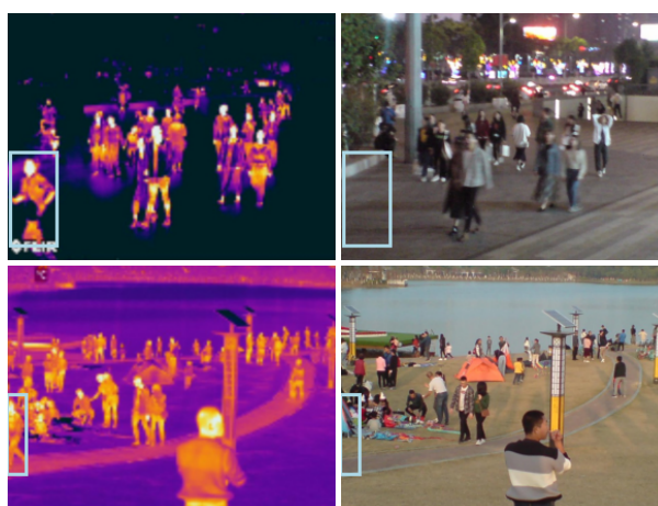
Figure 7: Two examples from the RGBT-CC dataset where a person is visible in one modality but not the other. It can be seen that this is due to the time-delayed capture of the images from both modalities.
