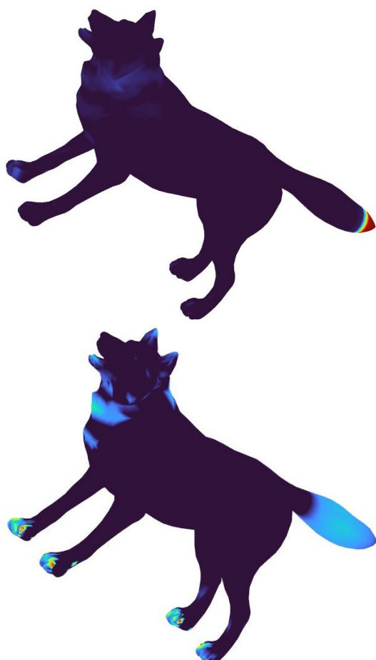
Figure 7: Geodesic Error Plot visualized as heat map on the shape itself; via Hamiltonian basis (top); via Laplace-Beltrami basis (bottom) for wolf mesh
