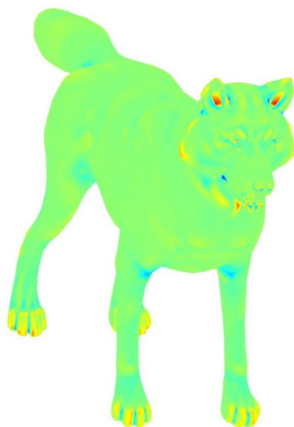
Figure 3: Gaussian Curvature visualized on wolf shape
