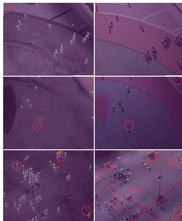
Figure 6: The annotations of the Drone-RGBT [Pen20] dataset are shown in yellow squares. It can be seen that the annotations were made on the basis of the thermal images. For better understanding, individuals have been encircled who are easily recognizable in the optical image, but have not been annotated. In the thermal image, on the other hand, it can be seen that precisely these individuals are difficult to recognize, which is probably why they were not annotated.
