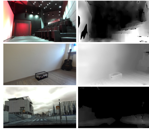
Figure 7: Experimental Setup : Selected measurement locations (left side) and their associated depth images (right side). Top: Indoor space of a Lab; Middle: Model vehicle in a residential building; Bottom: Outside in a moving vehicle
